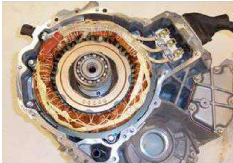
Figure 8: PMSM used in Toyota Prius
