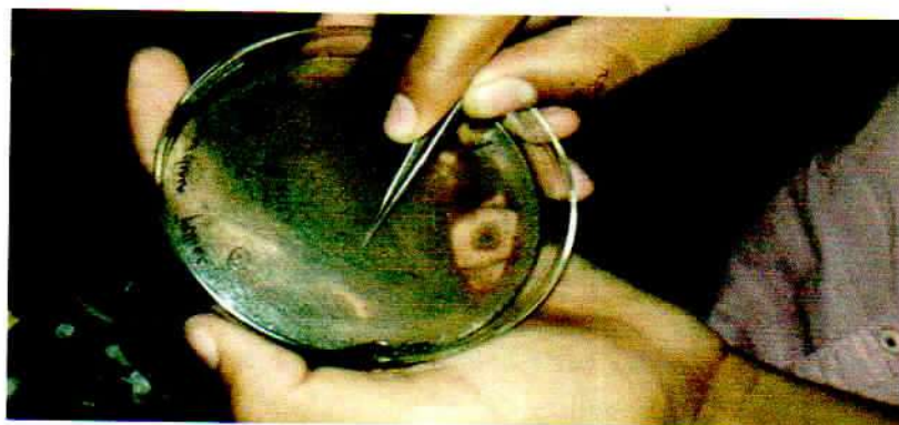
The so formed nanoparticles obtained from the dried plate using a sterile spatula
