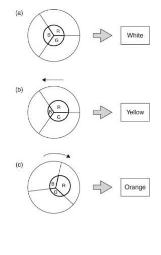
Burnham colorimeter with red, green, blue filters and aperture plate. (Different quantitites of R, G and B in mixture give white, yellow, orange and other colours.)
