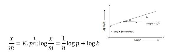
x represents the amount of gas adsorbed on the m gram of adsorbent, K and n are adsorption constants, 'p' is pressure n always greater than one. A major drawback of Freundlich adsorption isotherm it fails at high pressure. It could not explain the multi-layered adsorption process.
