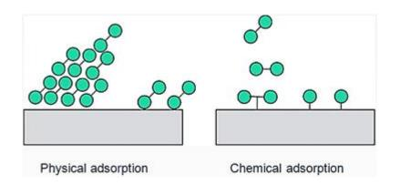
Adsorption constants are basically equilibrium constants. What it means is that they also follow or obey the van 't Hoff equation:  $\left(\frac{\partial \ln K}{\partial \frac{1}{T}}\right)_{\theta} = -\frac{\Delta H}{R}.$
