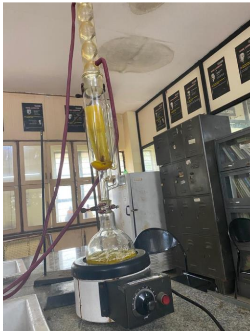
Fig:9 EXTRACTIN AND ISOLATON OF TURMERON USING SOXHLET APPARATUS
