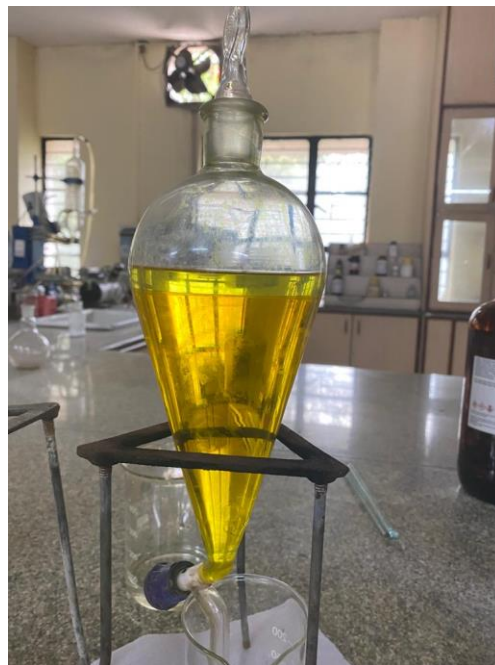
Fig:10 SEPARATION OF TURMERIC OIL USING SEPARATION FUNNELS
